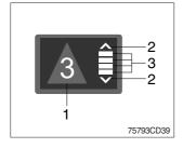
(1) The LCD can be used with the gear selector. It indicates speed and driving direction.
